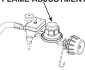
The regulator control valve is used to adjust the burner flame. Turning the control knob clockwise slowly will increase the burner flame and counter clockwise to decrease and shut the burner flame off.
